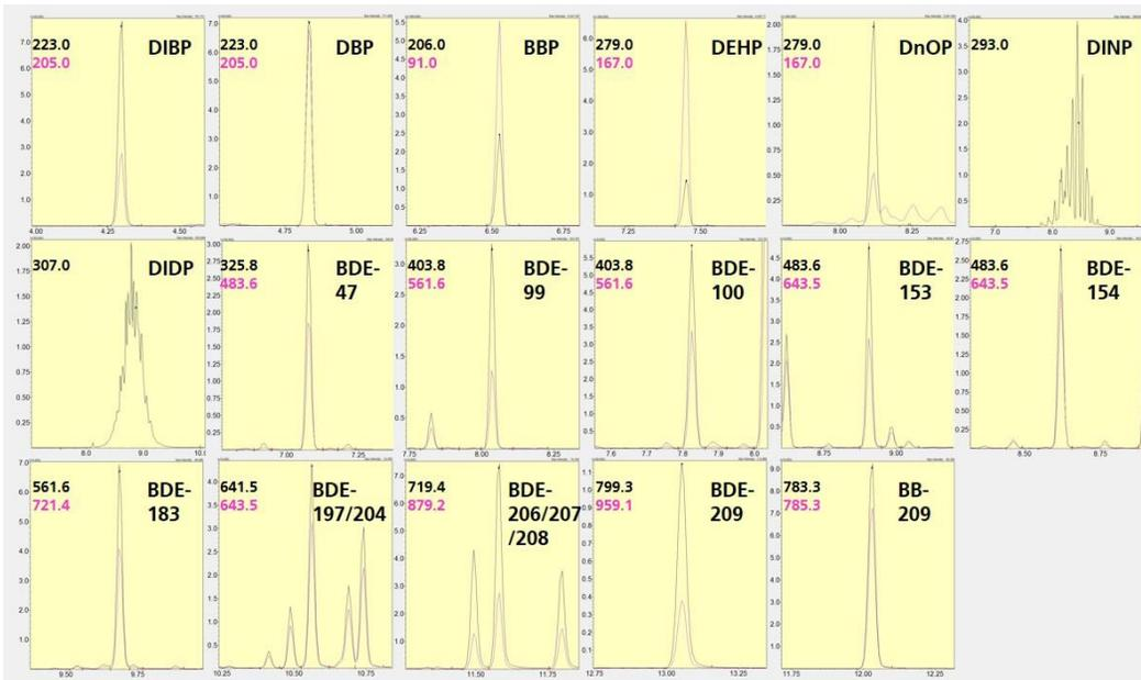
**Figure 3:** Chromatographic profile of the target compounds extracted from SIM chromatogram of the phthalate and PBDE standards. The primary SIM ions are shown in black, and the secondary reference ions are shown in pink.
