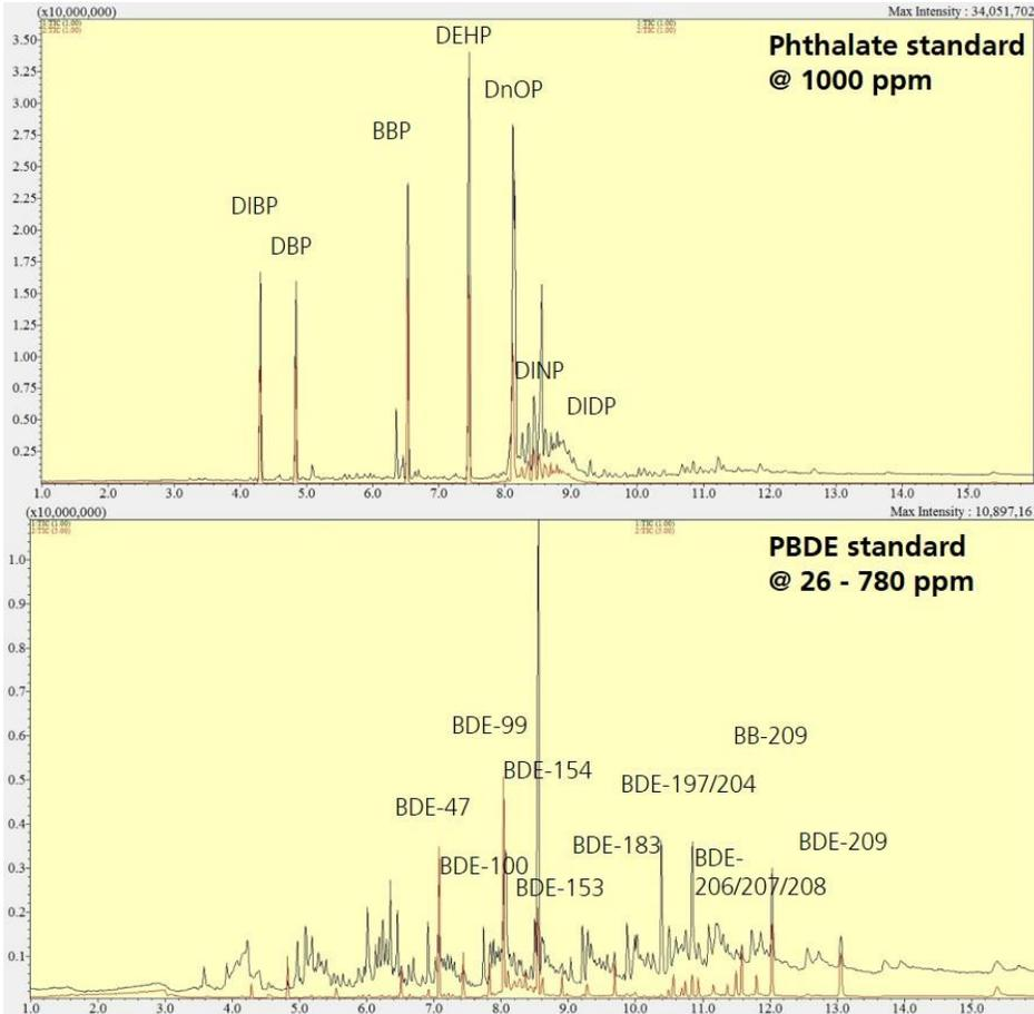
**Figure 2:** Total ion chromatograms (TIC) for the phthalate and PBDE standards, with full scan mode shown in black and SIM mode shown in red. Phthalate standard contains seven phthalates at 1000 ppm. The PBDE standard contains PBDEs and PBBs at various concentrations between 26 and 780 ppm.
