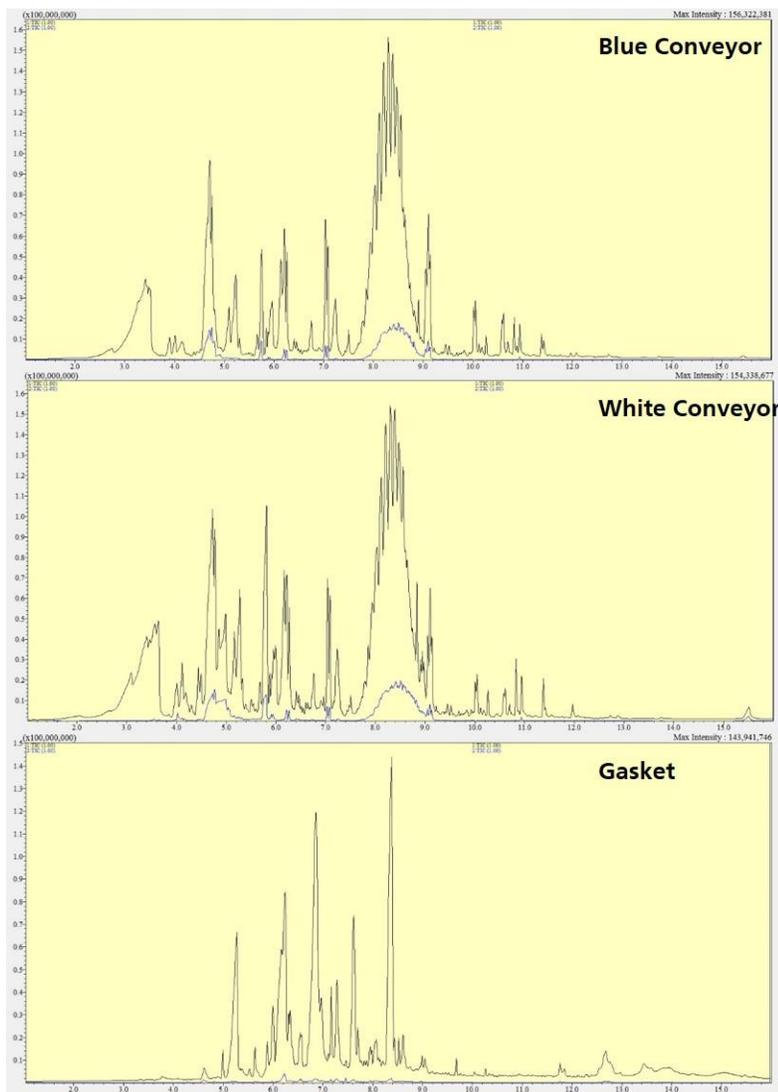
**Figure 4:** Total ion chromatogram from three samples - *Blue Conveyor*, *White Conveyor*, and *Gasket*, with full scan mode shown in black and selected ion monitoring (SIM) mode shown in blue. Note that the noise level in SIM mode is reduced significantly compared to full scan mode.
