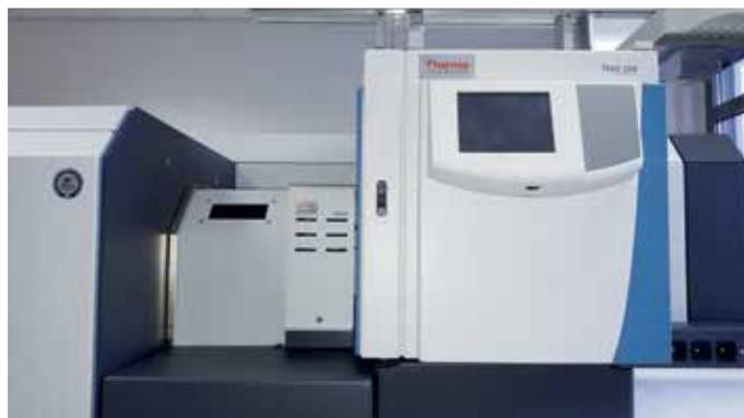
**Figure 10.** GCI 300 Interface between Trace 1310 GC and Neptune XT MC-ICP-MS.
