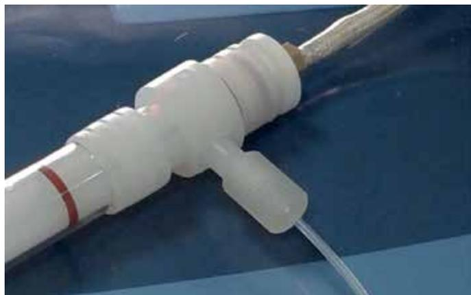
**Figure 1. Connection of GCI 300 Interface to semi-demountable torch and injector.** SF<sub>6</sub> gas could be added via the T-inlet.
