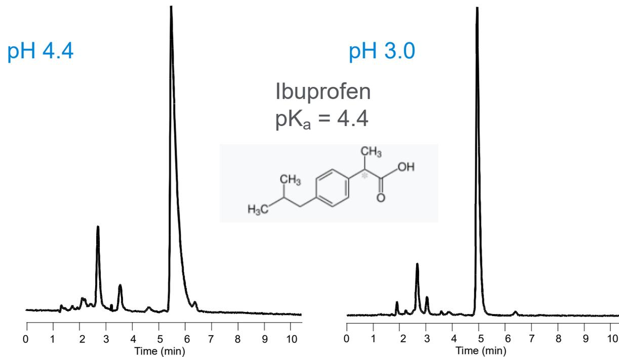
Column: ZORBAX SB-C8, 4.6 x 150 mm, 5 μm
