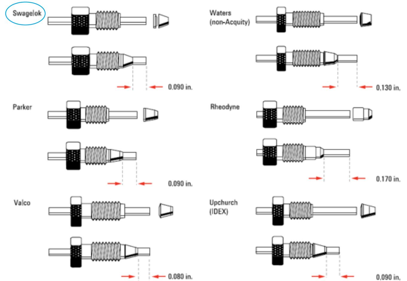
*Different fitting types have different stem lengths*
