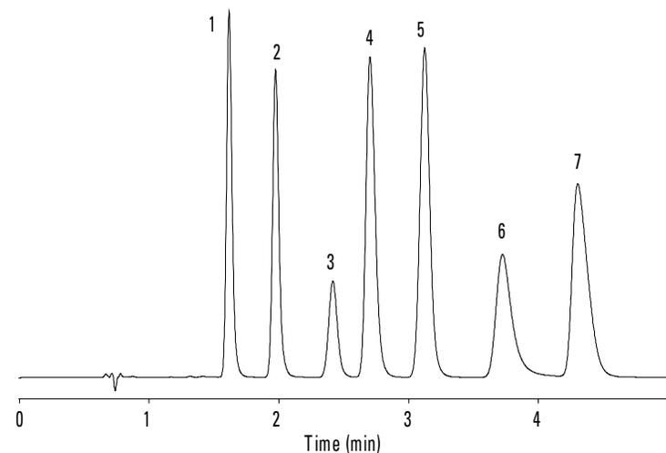
Column: ZORBAX Rapid Resolution Eclipse XDB-C8, 4.6 x 75 mm, 3.5  $\mu$ m      Mobile phase: 44% A : 56% methanol
