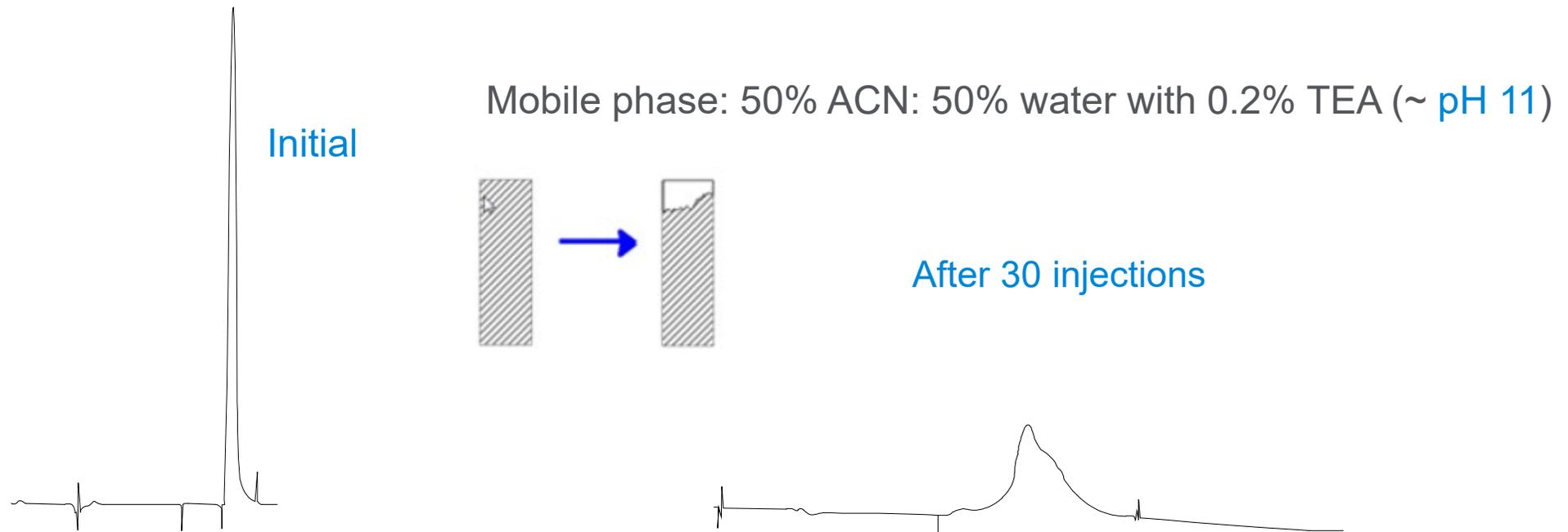
Multiple peak shape changes can be caused by the presence of a void in the column. In this case the void resulted from silica dissolved at high pH.
