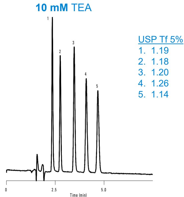
Columns: Eclipse XDB-C8, 4.6 x 150 mm, 5  $\mu$ m    Mobile phase: 85% 25 mM Na<sub>2</sub>HPO<sub>4</sub> : 15% ACN    pH: 7    Flow rate: 1.0 mL/min.
