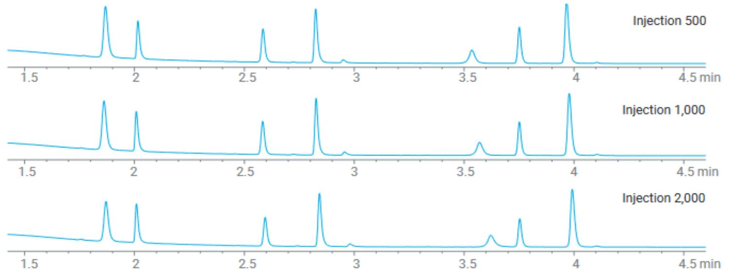
After 2,000 injections at pH 10, InfinityLab Poroshell 120 HPH-C18 showed no change in performance.
