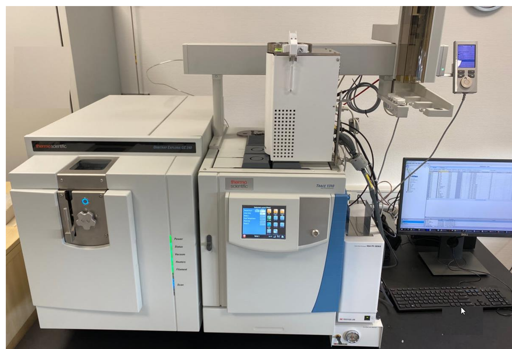
Figure 1. Orbitrap Exploris GC 240 with Frontier multi shot pyrolyzer installed on GC.
