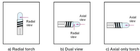
Figure 1. Plasma viewing options in ICP-OES instruments.
