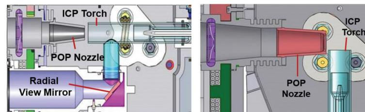
Figure 2. Schematic of the POP tubes for Duo (above) and Radial (below) instruments.
