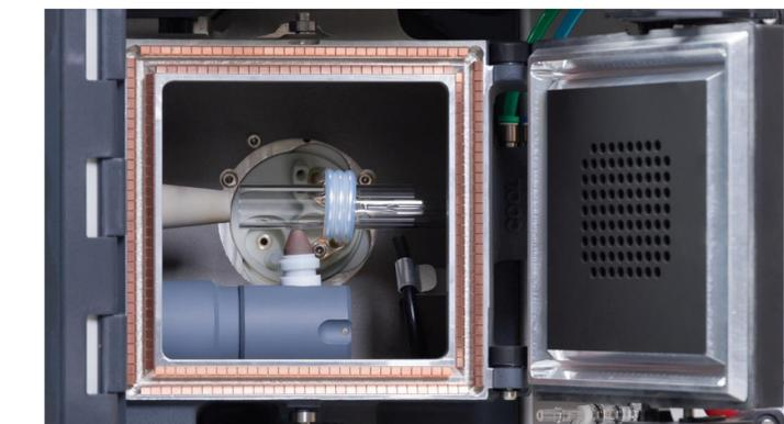
Figure 3. The torch box of a dual view iCAP 7000 Plus Series ICP-OES, showing the two POP plasma interfaces.
