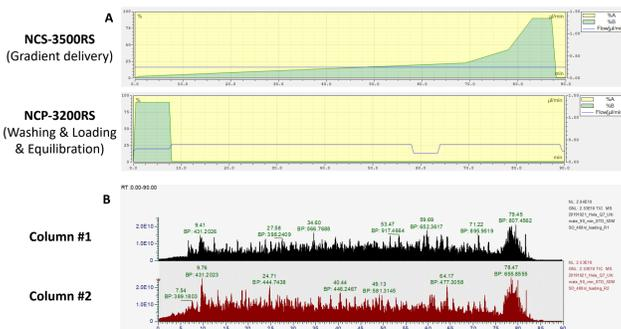
**Figure 7. The operation principle of tandem nanoLC pre-concentration injection setup. The NCS-3500RS pump delivers gradient for sample separation on columns 1 or 2, while NCP-3200RS pump, loading pump and WPS-3000TPL RS autosampler are used for offline trap column and analytical column washing and equilibration, sample injection and loading.**
