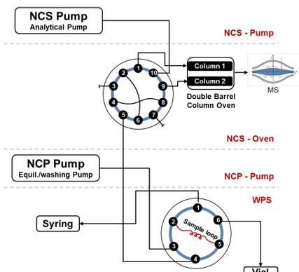
**Figure 4. Tandem nanoLC pre-concentration injection fluidics setup that requires two 2-position 10-port valves and loading pump integrated into NCS-3500RS module for sample separation on column 1 and column 2.**
