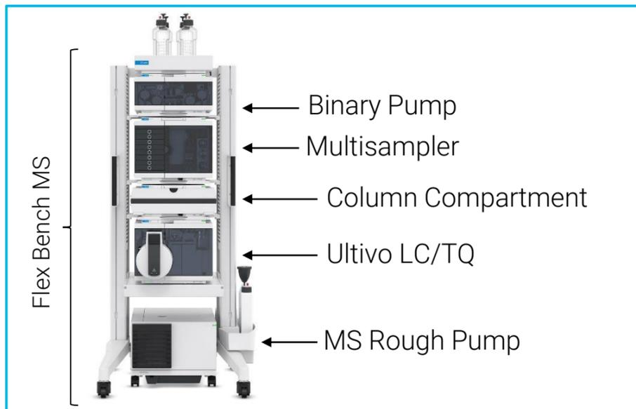
Figure 1. Ultivo triple quadrupole LC/MS system
