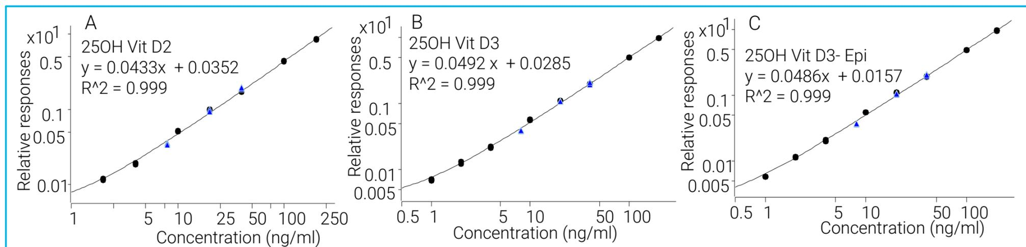
Figure 4. The calibration; A: 25(OH)D2, B: 25(OH)D3, & C:25(OH)D3-epi. The three QC levels are marked in a blue triangle. (calibration model Type: Linear, Origin: Ignore, Weight: 1/x)
