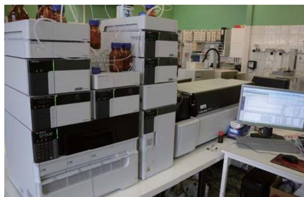
Fig. 1 Shimadzu UHPLC-MS/MS Nexera-8040 system
