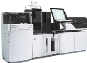
CLAM-2040 is an online automated sample preparation module that brings LC/MS smoothly into your laboratory. The CLAM-2040 accompanies you on most of the analytical workflow and improves your overall throughput by drastically reducing the sample preparation time. Simply place the blood tubes in position and the CLAM-2040 performs the next steps automatically, from sample extraction, up to the LCMS analysis and data processing.
