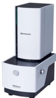
The SPM-Nanoa scanning probe microscope provides high-resolution observations, features a low-noise detection optical mechanism, and automates optical adjustments and the work of setting the observation conditions. Even users unfamiliar with the operating procedures can easily acquire high-resolution observation data. It will contribute to the evaluation of, and research into, cutting-edge nano materials as a mid-range scanning probe microscope (SPM).
