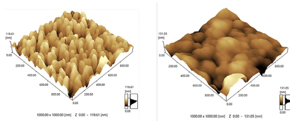
Figure 5: Left: Baseline Ag nanorods topography correlative to the SEM imaging A in Figure 1. Right: Local mapping of topography for Ag Oxidized Nanorods after sitting in water for 2 hours.
