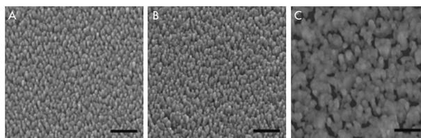
Figure 1. SEM image of Ag nanorods after exposure to (A) air, (B) degassed deionized water, and (C) non-degassed deionized water for 168 hours. The scale bars are 500 nm.
