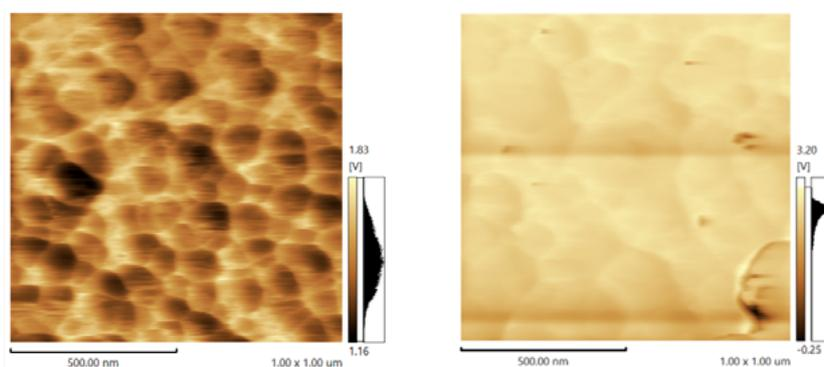
Figure 6: Left: Ag nanorods surface potential contour map taken immediately after removal from vacuum. Right: Ag nanorod surface potential contour map taken after submersion in non-degassed water for two hours.
