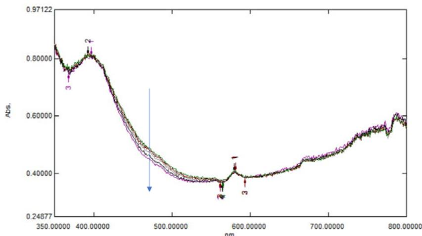
Figure 3. Time resolved UV-Vis reflection spectra for a Ag nanorod sample exposed to non-degassed deionized water. Spectra are taken every 10 minutes over one hour and progress in the direction of the arrow.
