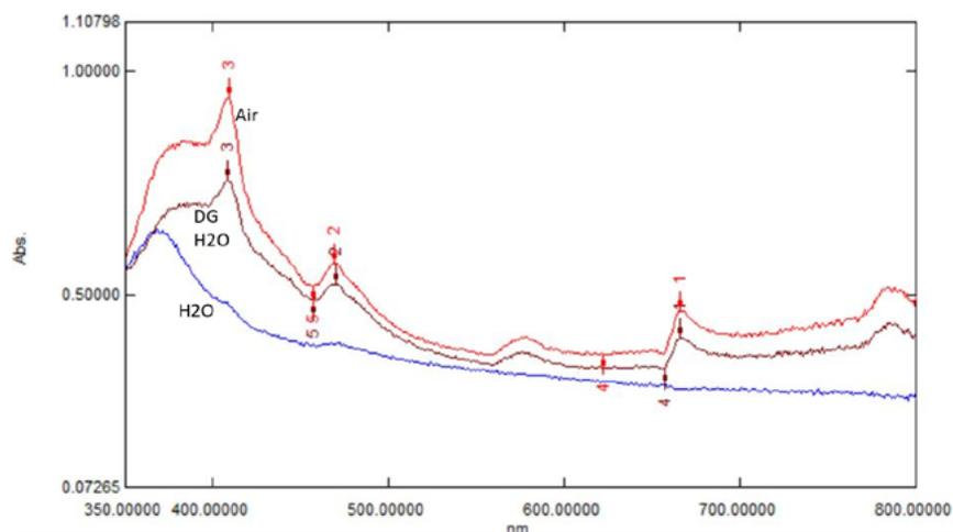
Figure 2. UV-Vis reflection spectra for Ag nanorod samples exposed to varied conditions for 12 hours.
