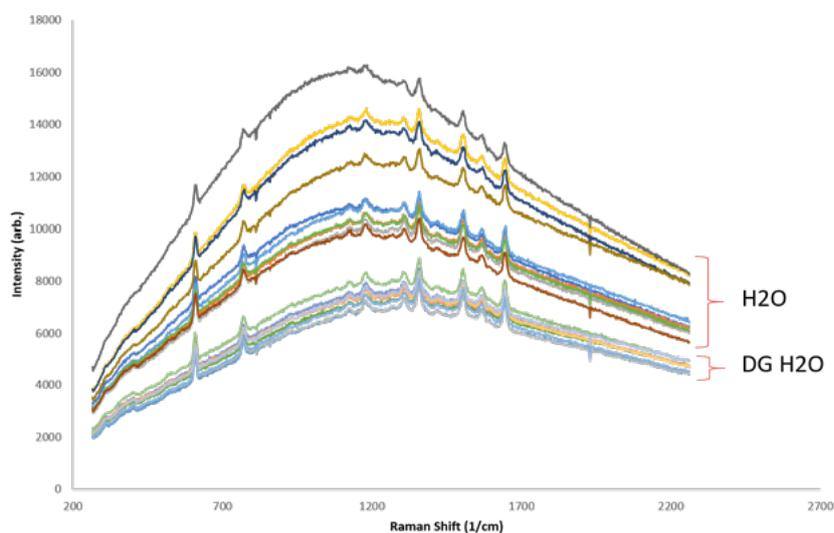
Figure 4. Raman spectra of Ag nanorods sensitized with R6G solution in non-degassed de-ionized water, labeled H<sub>2</sub>O in the Figure, and degassed water, labeled DG H<sub>2</sub>O in the Figure.
