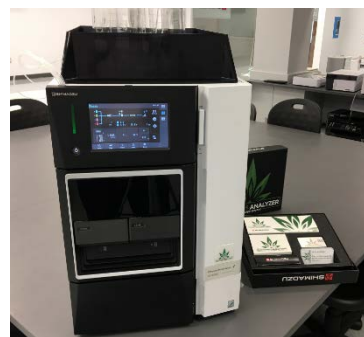
Shimadzu Cannabis Analyzer for Potency analyzes 11 cannabinoids
