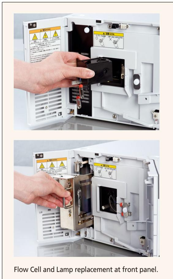
Flow Cell and Lamp replacement at front panel.
