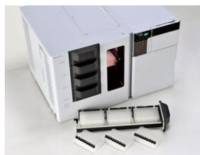
**The Rack Changer II** accommodates up to 12 sample plates (96 well, 384 well, vial plates) to allow up to 4608 samples to be continuously analyzed unattended. It incorporates fine temperature control with a cooling function (4 to 40°C) to minimize sample degradation during the process.
