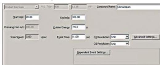
Fig. 2 User Interface of MRM-Product Ion Scan setting at LabSolutions software
