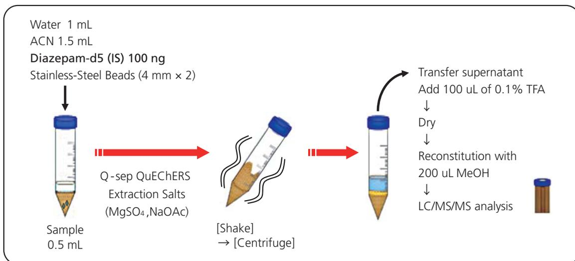
Fig. 1 Scheme of the modified QuEChERS procedure
