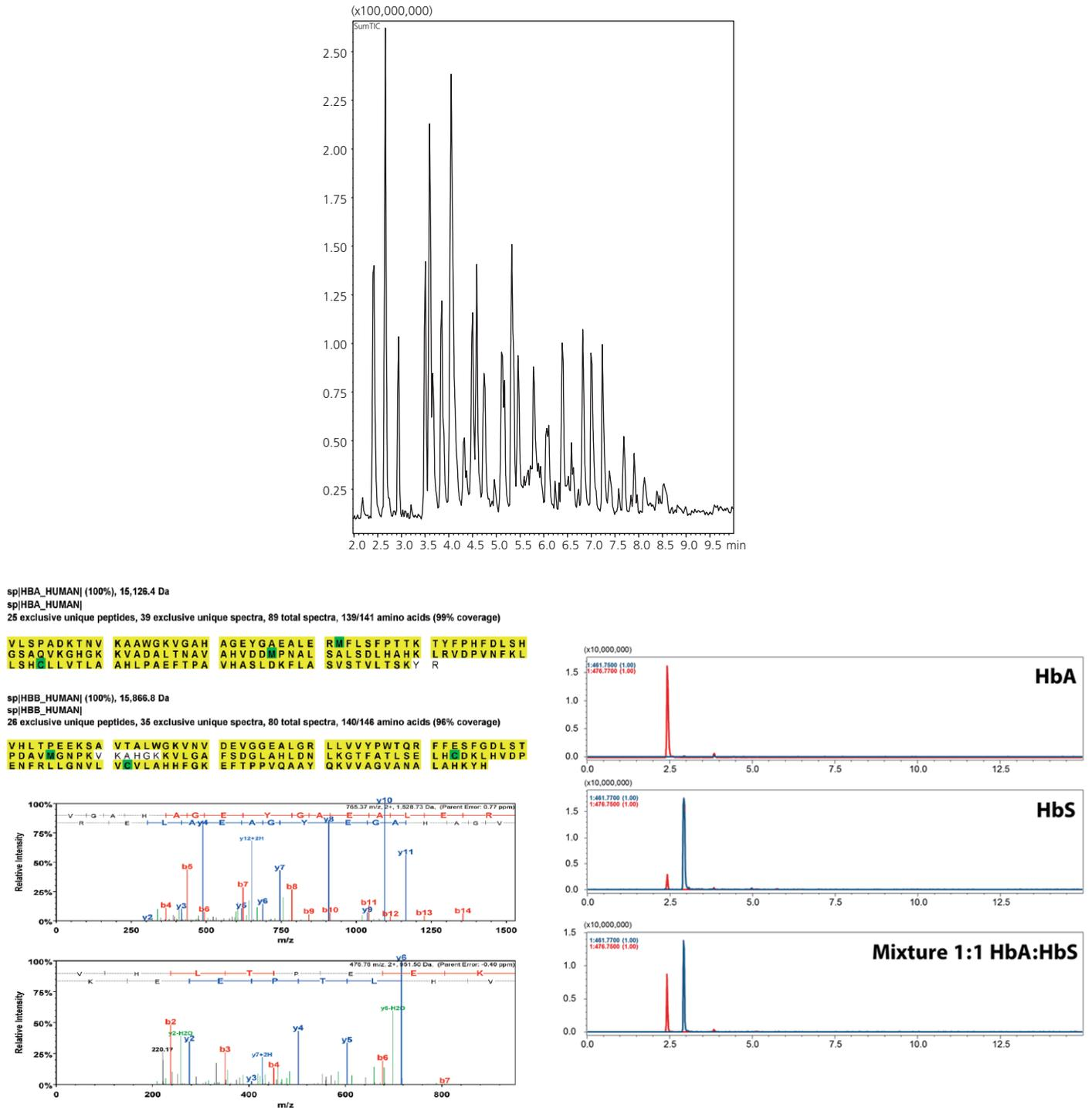
Figure 1. Data dependent discovery (DDA) of protein isoforms. Digestion using the Perfinity Workstation (PWS) was optimized for hemoglobin variants (4 minute digestion at 40°C) and mixtures were analyzed using the LCMS IT-TOF with a top 3 approach on a 15-minute gradient at 0.5 mL/min. Coverage at 5 % protein FDR was approaching 100 %, and isoform peptides were identified.
