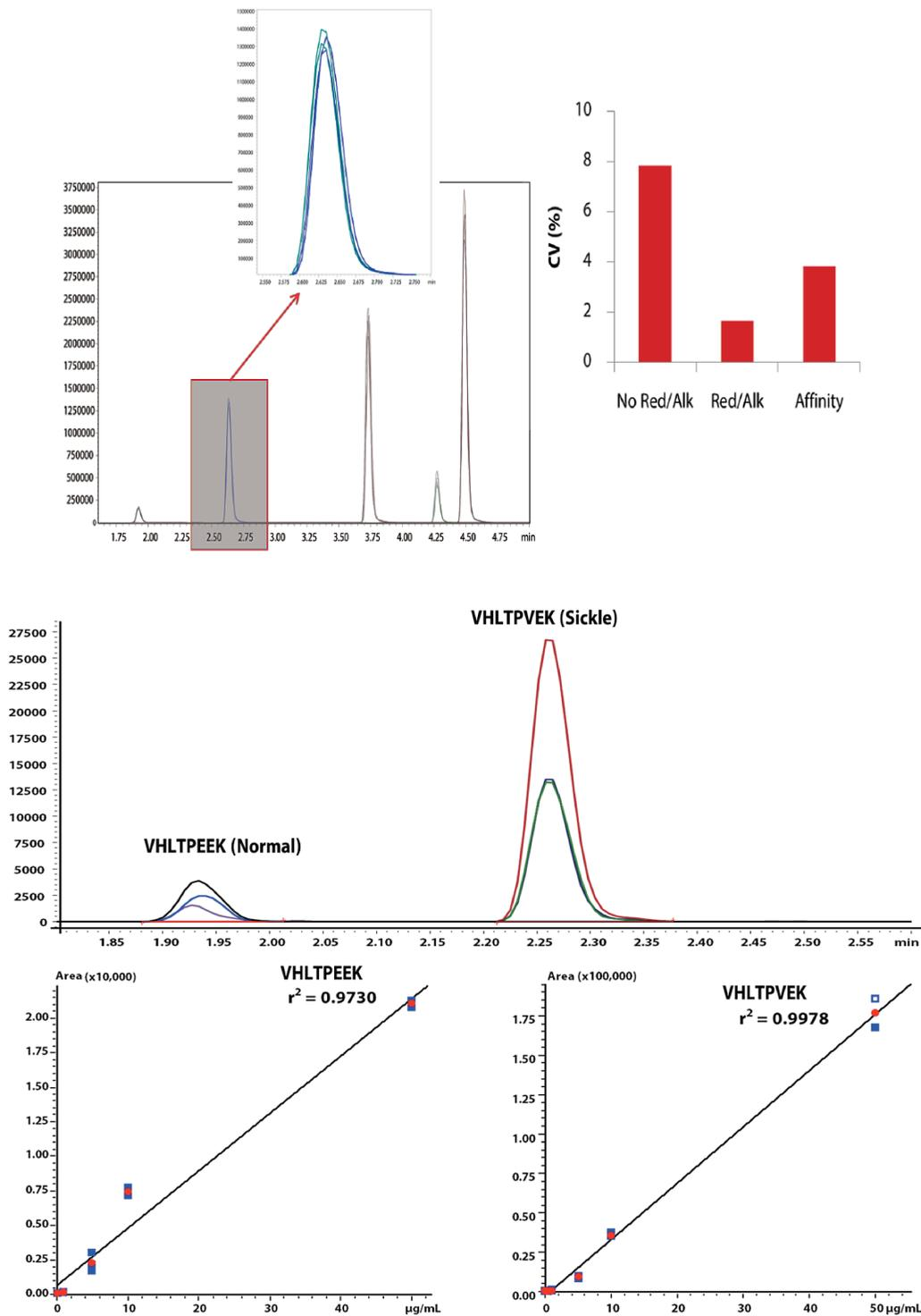
Figure 2. Reproducible, accurate quantitative analysis of protein isoforms. Protein isoforms identified via DDA were analyzed using the PWS coupled to an LCMS-8050 using the digestion and affinity parameters optimized in previous experiments. The sickle and wild type peptides were resolved and quantified using a 5 minute gradient at 0.5 mL/min. CVs for the acquisition were below 8 % for all experiments.
