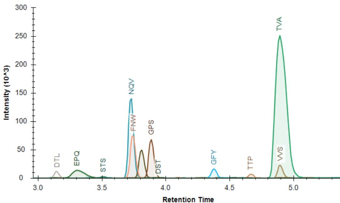
**Figure 3. Rapid immuno-MRM of human IgG.** Samples were affinity captured using a Protein G column, digested and analyzed using a Perfinity Workstation coupled to an LCMS-8050 triple quadrupole. Target peptides and transitions were selected using Skyline; source and CID conditions were optimized manually. A standard curve was generated and 12 peptides from the constant and variable regions of IgG were monitored.
