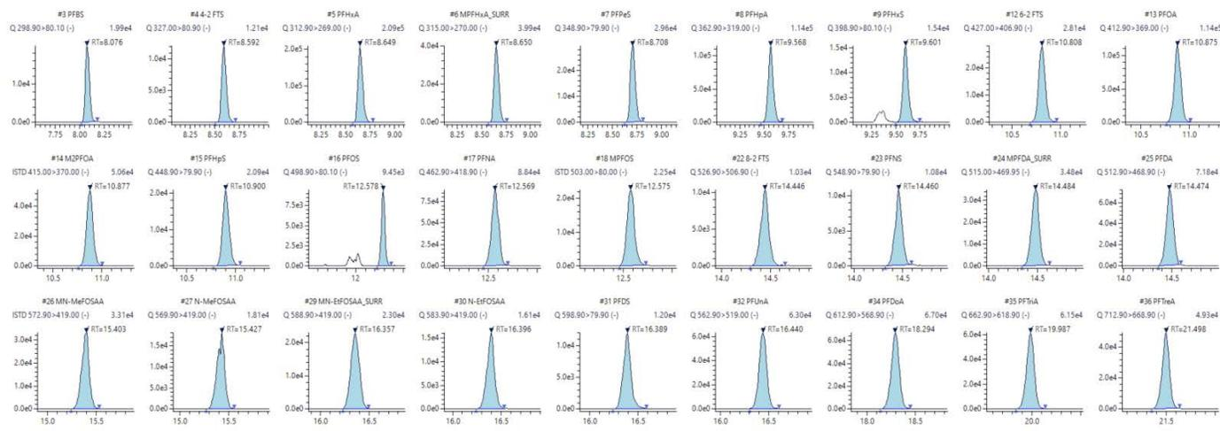
**Figure 2:** Chromatograms for all compounds at the Mid-Level Calibrator (20 ppb). Isomers of PFOS and PFHxS were detected and chromatographically separated
