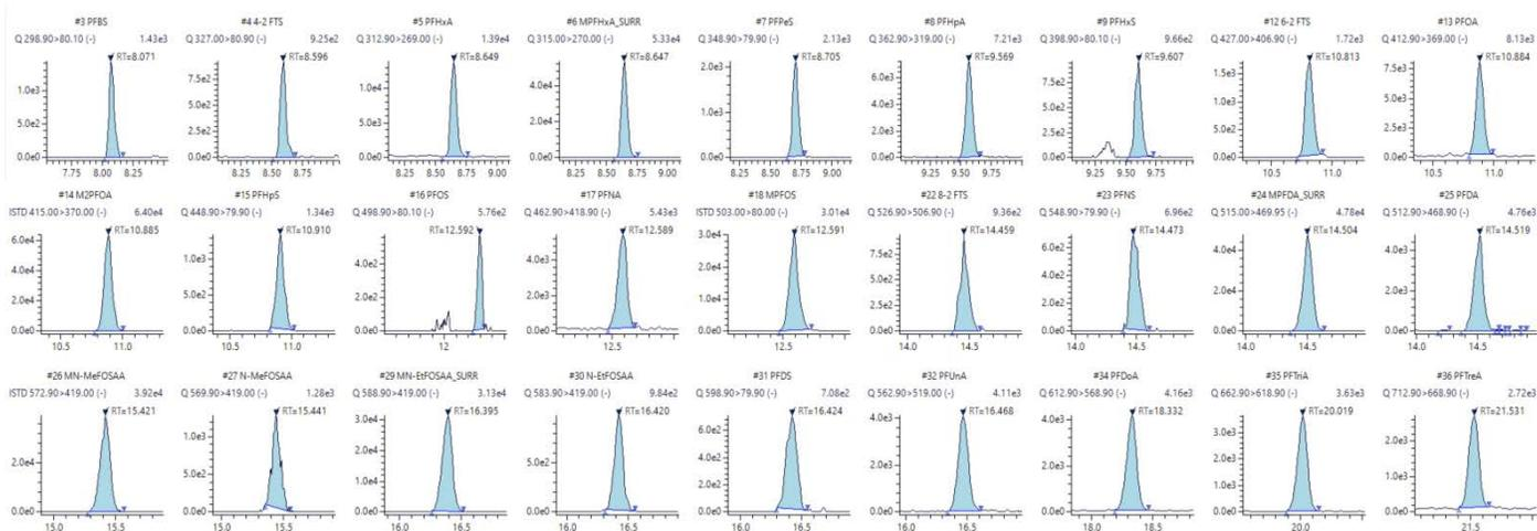
**Figure 4:** Chromatograms for all compounds for the MDL Study (5 ppt). Isomers of PFOS and PFHxS were detected and chromatographically separated
