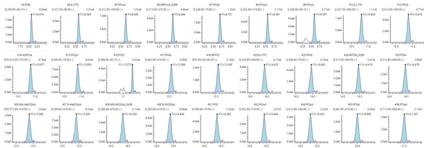
**Figure 3:** Chromatograms for all compounds at the ULOQ (100 ppb). Isomers of PFOS and PFHxS were detected and chromatographically separated
