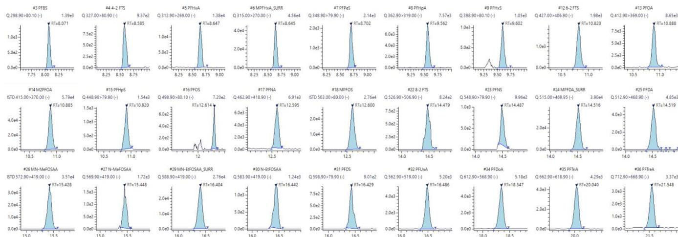
**Figure 1:** Chromatograms for all compounds at the LLOQ (1.25 ppb). Isomers of PFOS and PFHxS were detected and chromatographically separated
