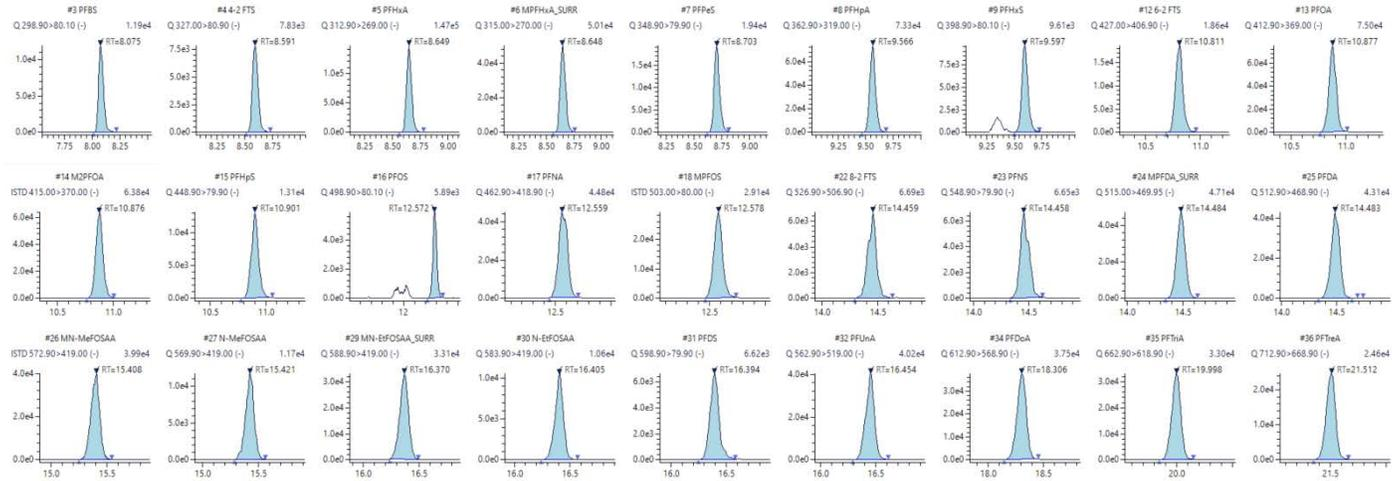
**Figure 5:** Chromatograms for all compounds for the Precision and Accuracy Study (60 ppt). Isomers of PFOS and PFHxS were detected and chromatographically separated
