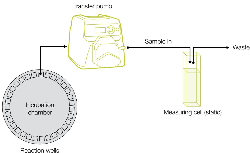
Figure 3. Hybrid discrete analyzer.
