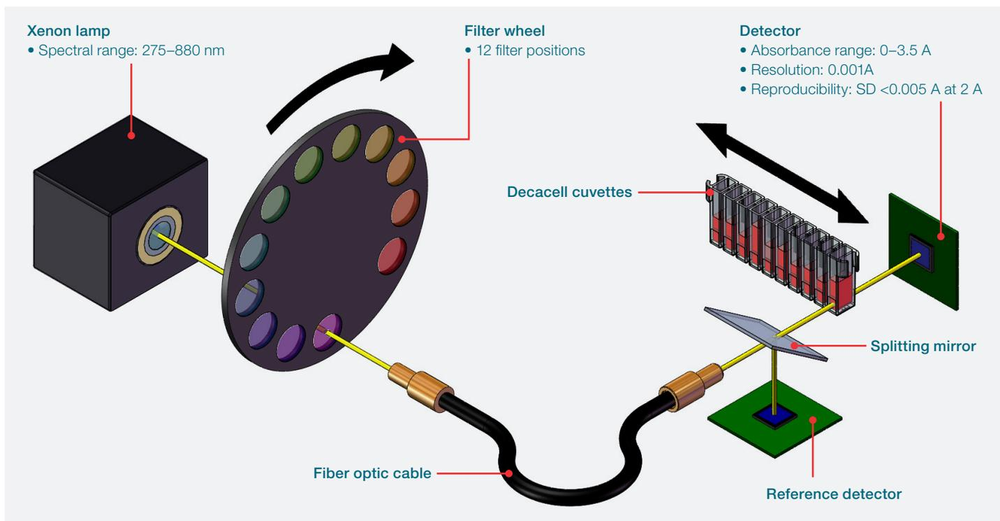
Figure 4. Gallery Discrete Analyzer—photometric measurement.
