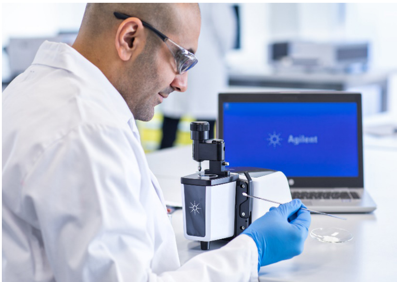
Figure 1. An Agilent Cary 630 FTIR spectrometer with a diamond ATR module is the ideal tool for the fast, easy analysis of nutrients in crop samples.
