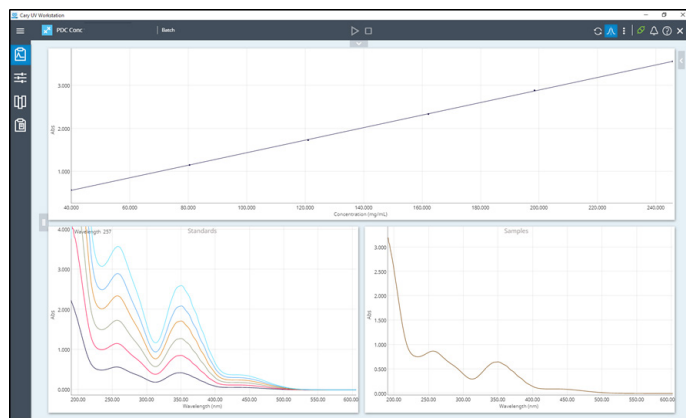
Figure 5. The absorbance spectra of the standards measured on the Cary 3500, and the calibration curve produced from the absorbance at 257 nm. The sample absorbance scan is shown in the bottom-right window.
