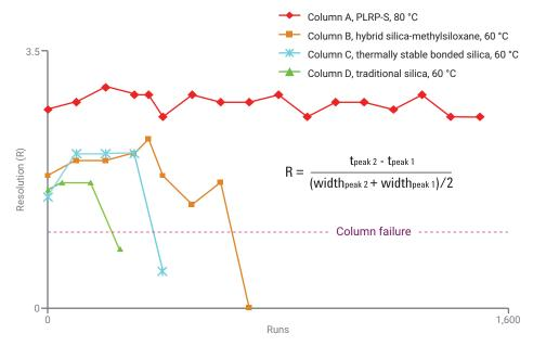
Figure 3. Column lifetimes at elevated temperature, plot of numbers of cycles versus resolution.
