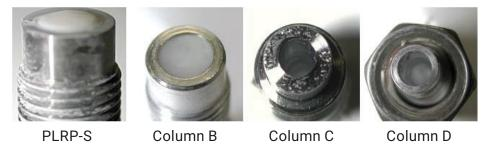
**Figure 4.** Column inlet photographs at the end of the stability trial. PLRP-S media remains intact at higher temperatures, keeping oligo samples free of dissolved media.
