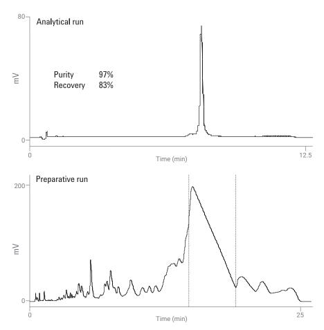
**Figure 2.** Purification of a 25mer trityl-off and analytical quantitation of fraction. Higher purity levels. 100 nmol purification: 25mer trityl-off, 4.6 × 50 mm PLRP-S column.
