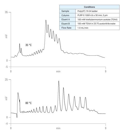
Figure 1. Reversed-phase separation of Poly(dT) 19-24 ladder at 35 and 80 °C.
