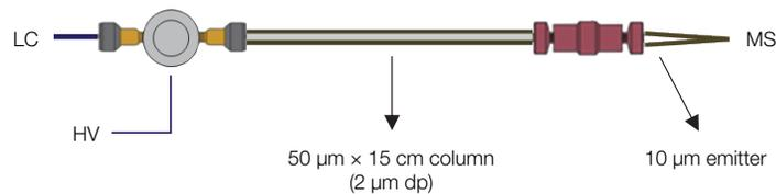
Figure 1. Direct injection workflow using 1,500 bar for sample loading to increase sample throughput
