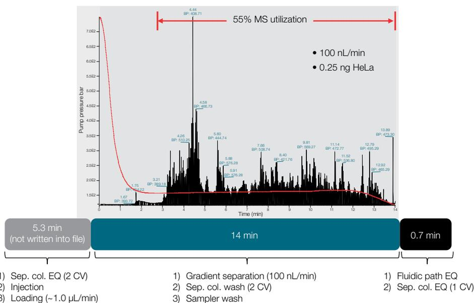
Figure 3. High-throughput method highlight. The 20-min cycle time with 11 min elution window (72 samples/day) enables 55% MS utilization through parallel gradient separation and sampler washing.
