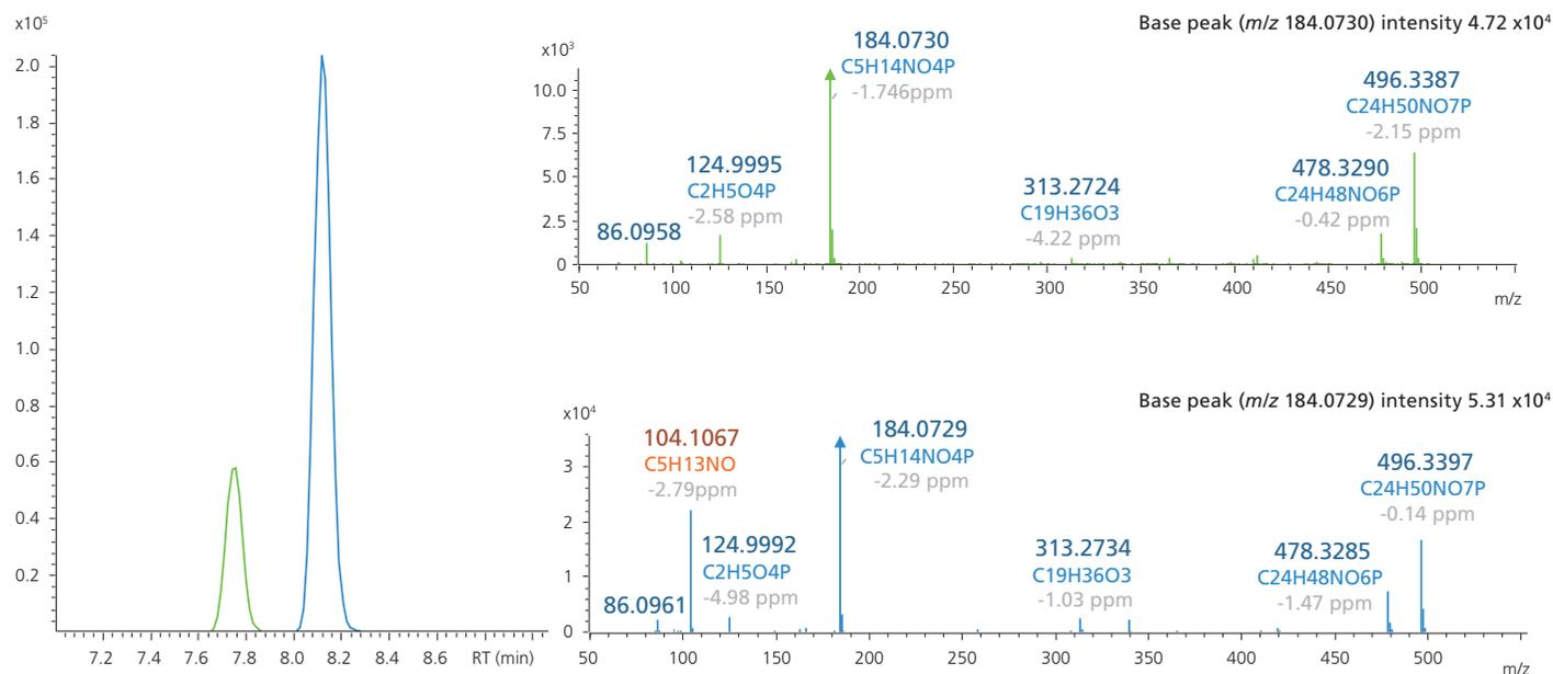
Figure 6. MS chromatogram for  $m/z$  496.3398  $\pm$  5ppm corresponding to LPC 16:0 *sn-1* and *sn-2* isoforms. Average MS/MS spectra shown for each peak (FWHM). The fragment at  $m/z$  104 is a characterized fragment of the *sn-1* isoform known to exceed a 30 fold difference in intensity relative to the same ion in the *sn-2* isoform (Han and Gross 1996). Neutral formulae for each fragment are shown.
