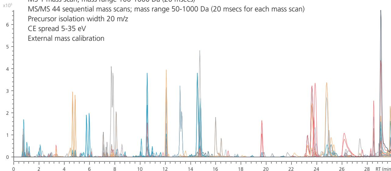
Figure 1. HRAM mass chromatograms of 627 components detected in the QC (5ppm extraction window).
