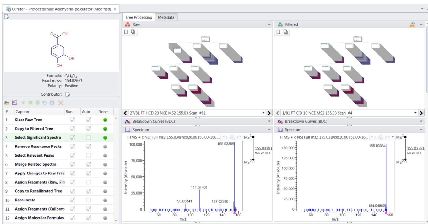
**Figure 5. Spectral library curation tools provided by Mass Frontier software.** Curator, part of Mass Frontier software, allows you to create your own high-quality spectral libraries; the left panels show the raw and uncurated data, and the right panel shows the filtered, curated data.
