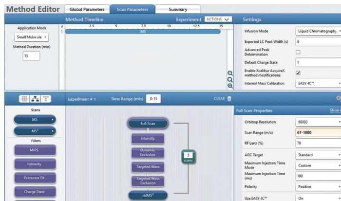
**Figure 4. Method Editor window used to setup the mass spectrometer parameters.** Plug-and-play nodes enable users to easily setup and customize the analysis to maximize data quality and Instrument performance. In addition to the templates, intuitive tuning and simplified calibration across the mass range and polarity modes add to usability, data quality, and sample throughput.
