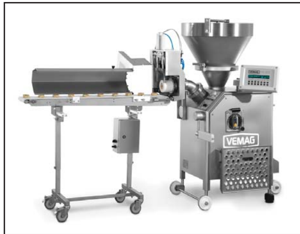
Robot 500 dough portioner with pneumatic cutter 811
