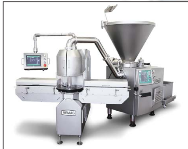
FKF II. – The can filling system
