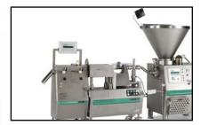
Line for grinding and separating meat for processing, consisting of ROBOT HP15C vacuum filler, separation grinder 982 and automatic separation valve
