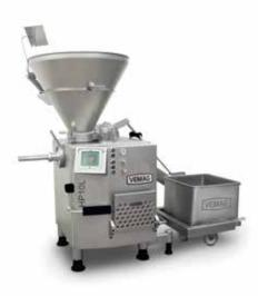
The HP10L is the linking specialist with double screws for fl exible use. The solution for all fi lling tasks encountered in sausage production without a grinder. Your skill with casing holding devices or VEMAG fl exible sausage lines becomes particularly evident. As a result, linking and portioning, even of soft products, is child's play.
