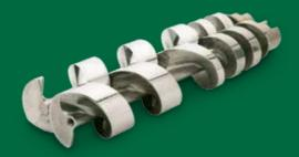
The double screws are at the heart of VEMAG filling machines. The double screws transport even raw materials containing large pieces especially gently all the way from the inlet to the outlet of the machine without a compression zone. The raw material is transported gently and without stress, making your products
