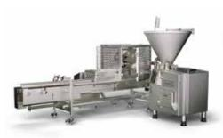
The roller filling head 863 portions rye doughs, wholemeal doughs, gluten-free doughs and other mixtures directly into moulds in a clean process and with a high degree of weight accuracy. It is optimally designed for fully automated industrial portioning of french bread or artisan portioning of french bread using a safety table. The roller filling head 863 achieves an output of up to 50 portions per minute for an extremely efficient production process.
