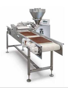
The sheeting horn is used wherever soft doughs and mixtures need portioning with a high degree of accuracy and positioning directly on sheets or flat products, such as tray bakes, toppings or fillings. The sheeting horn is fitted with a pneumatically operated roller closure and can be adjusted to specific requirements, such as different sheet sizes.
