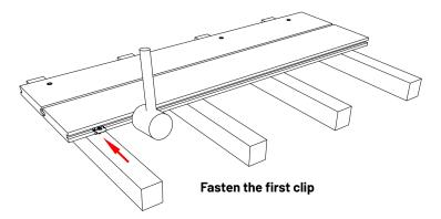
• Move to the opposite end of the board, ensuring suitable engagement of the board with the previous row of clips, and fasten a clip in the final position, locking the board into place.
