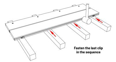
• Fasten the remainder of clips between the first and last clip ensuring the board is correctly positioned relative to the previous row clips.
