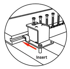
• Fasten the clip into place by installing the screw until it is fully seated on the clip. Ensure the head of the screw clears the tool and the board.
