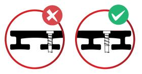
Avoid driving the top fixing screws through the web of the profile shape, this would cause cracking.
