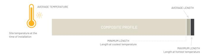
If the site is hotter than the expected average temperature, then the boards are expected to contract when the temperature drops to the average and the installed gap must be adjusted narrower accordingly.
