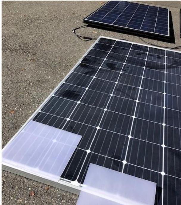
Figure 6. Opaque plastic sheets covering sections of the PV module to control PV Power input during testing
