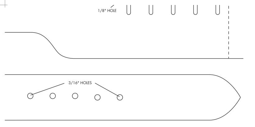
NOTE: CUT A STRIP 3" WIDE AND 8" LONGER THAN WAIST SIZE. USE TEMPLATES TO FORM THE BUCKLE END AND TONGUE. LOCATE SLOTS FOR BULLET LOOPS AS NEEDED
