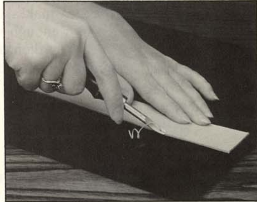
Hold an edge beveler at an angle to trim the edge.
