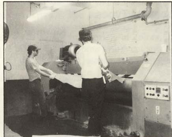
This setting machine smooths out the damp leather. Courtesy of Hermann Oak Leather Company
