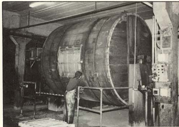
Drums which turn and add chemicals to the skin Courtesy of Hermann Oak Leather Company
