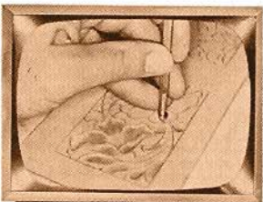
Figure 7. USE PEAR SHADER TOOL #206.
