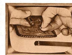
Figure 12. SET STUD AND EYELET OF SNAP.
