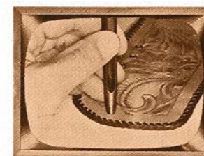
Figure 10. PUNCH BOTH SNAP HOLES.
