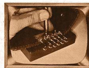
Figure 8. INSTALL AND SET EYELETS.
