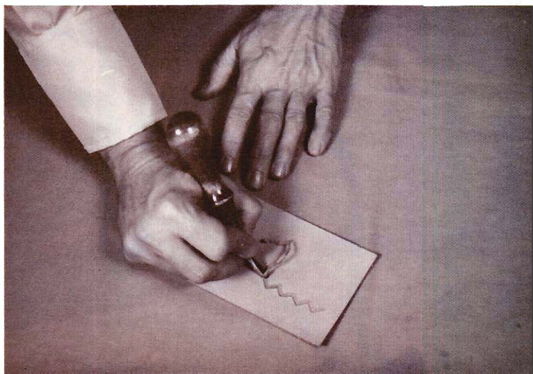
Step 4. To facilitate control of gouge when working on intricate cuts, you may wish to grasp shaft of gouge near cutting tip as shown.
