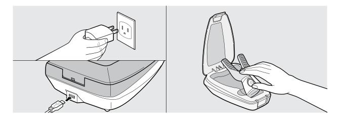
**5.1.1.** Power the Charging Case by connecting the USB Charging Cable to an electrical source.
