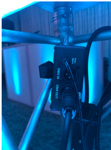
Wireless Di-Fi DMX Transmitter & Furman Box inside the trussing
