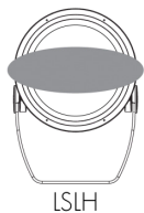
LSLH - Linear spread lens horizontal distribution
