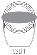
LSLH - Linear spread lens horizontal distribution
