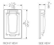
DRG IU - Ground Fault Duplex Receptacle (While in Use)
