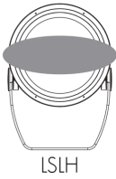
LSLH - Linear spread lens horizontal distribution
