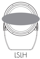
LSLH - Linear spread lens horizontal distribution
