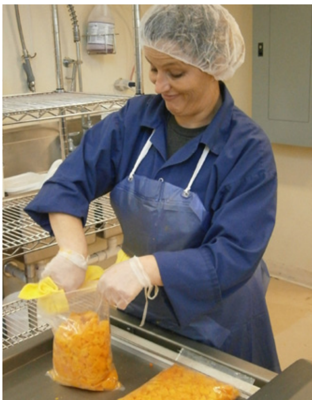
Vacuum-packing squash before freezing. Photo courtesy of Mission Mountain Food Processing Center.
