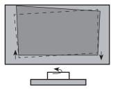
If the bottom of the image is lower on the right and higher on the left, rotate the device clockwise.
