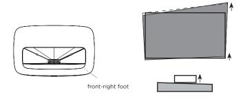
2. Now, rotate the Laser Cinema counterclockwise so that the bottom of the image is parallel with the screen.
