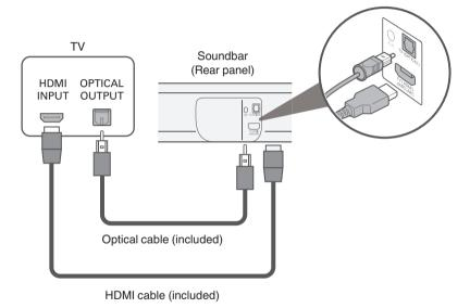
• Line up the optical cable with the shape of the terminal to insert.
