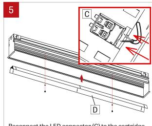
Reconnect the LED connector (C) to the cartridge (D). Reinstall the cartridge (D) by **using a screw with plastic washer. Do not apply too much pressure.**
