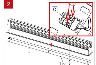
Disconnect LED molex connector (C) by taking a pointed object and pressing on the two tabs on the top. Unscrew the cartridge (D) and place it in a safe place.
