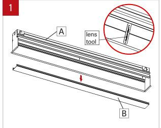
Make sure the power to the fixure (A) is turned off. Remove the lens (B) with the included lens tool.
