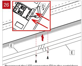
Reconnect the LED connector (D) to the cartridges (E) correctly. Reinstall the cartridges (E) by **using a screw with plastic washer. Do not apply too much pressure.**
