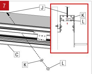
Insert fixture (C) into pre-cut hole in drywall, aligning threaded rods (J) with holes in top of fixture (C). Put washers (K) and tighten nuts (L) to secure the fixture (C).
