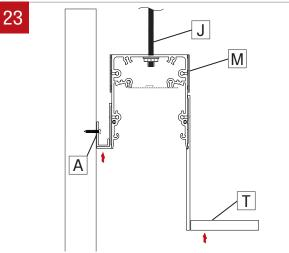
Adjust the second fixture (M) to the threaded rods (J). On wall side, the fixture (M) must touch the J-Bar (A). On ceiling side, flange need to be flush with the tile (T).
