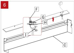
Install power cable (F) (by other) through the BX connector (G) (by other) and install onto the power plate (H) provided. Make electrical connections between power cable (F) and fixture cables using electrical marettes (I). Reinstall the power plate (H) to the fixture (C).
