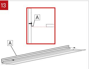
Locate J-Bar (A) position using provided client drawing. Install wall brackets to wall. Align with structural stud or use drywall anchors when needed. For sleeve adjustment, please refer to end-sleeve installation sheet.
