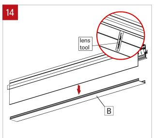
Remove lens (B) from all the fixtures in the run with the included lens tool.
