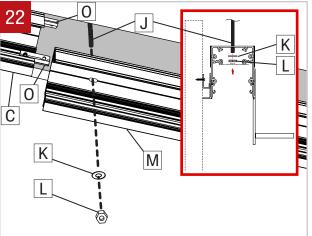
Insert the second fixture (M) into pre-cut hole in drywall, aligning threaded rods (J) with holes in top of fixture (M) and with the first fixture (C) with aligning brackets (O). Put washers (K) and tighten nuts (L) to secure the fixture (M).
