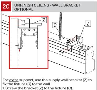
2. Screw the fixture(C) with the bracket(Z) to the wall.
