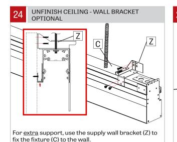
2. Screw the fixture(C) with the bracket(Z) to the wall.
