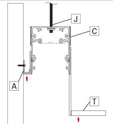
Adjust the fixture (C) to the threaded rods (J). On wall side, the fixture (C) must touch the J-Bar (A). On ceiling side, flange need to be flush with the tile (T).
