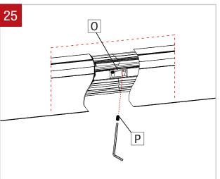
Tighten the set screws (P) on both joining brackets (O) using Allen Key to secure the fixtures together.
