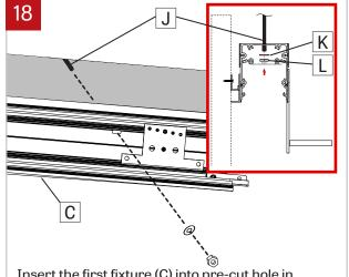
Insert the first fixture (C) into pre-cut hole in drywall, aligning threaded rods (J) with holes in top of fixture (C). Put washers (K) and tighten nuts (L) to secure the fixture (C).
