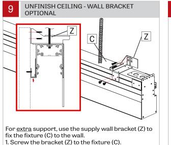
2. Screw the fixture(C) with the bracket(Z) to the wall.
