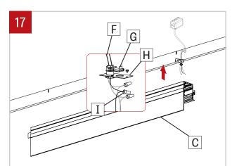
Install power cable (F) (by other) through the BX connector (G) (by other) and install onto the power plate (H) provided. Make electrical connections between power cable (F) and first fixture cables using electrical marettes (I). Reinstall the power plate (H) to the first fixture (C).
