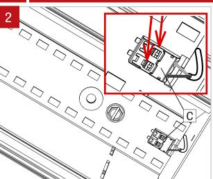
Disconnect LED molex connector (C) by taking a pointed object and pressing on the two tabs on the top.
