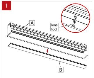
Make sure the power to the fixure (A) is turned off. Remove the lens (B) with the included lens tool.
