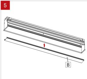
Reinstall the lens (B) back in place.
