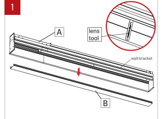
Make sure the power to the fixure (A) is turned off. Remove the lens (B) on the fixture (A) with the included lens tool.
