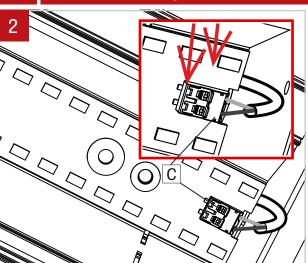
Disconnect LED molex connector (C) on the fixture's cartridge by taking a pointed object and pressing on the two tabs on the top.
