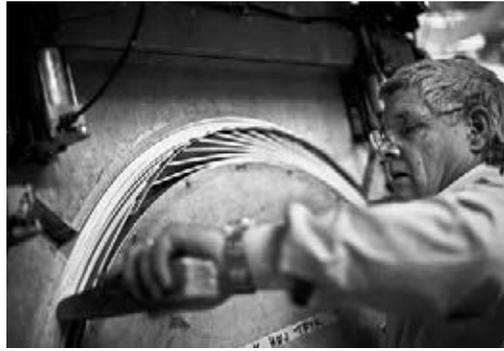
Laminating is possible because wood is flexible and thin pieces are easily bent. It is the technique of slicing up wood into thin pieces and gluing them together to form a new shape.
