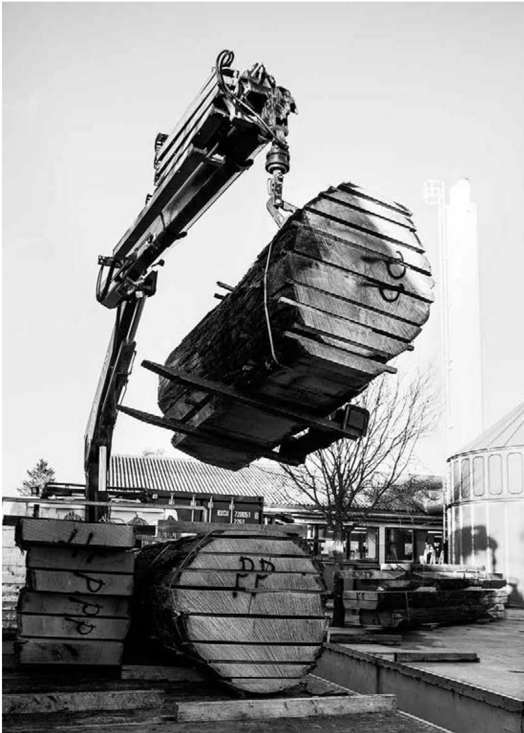
Whenever shelter trees are felled we take them immediately to the saw mill to be cut into 3, 4 and 5 inch planks. The freshly cut planks are then brought directly to our workshop. While the planks are still naturally moist we cut out and pair the raw pieces needed for a particular chair.
