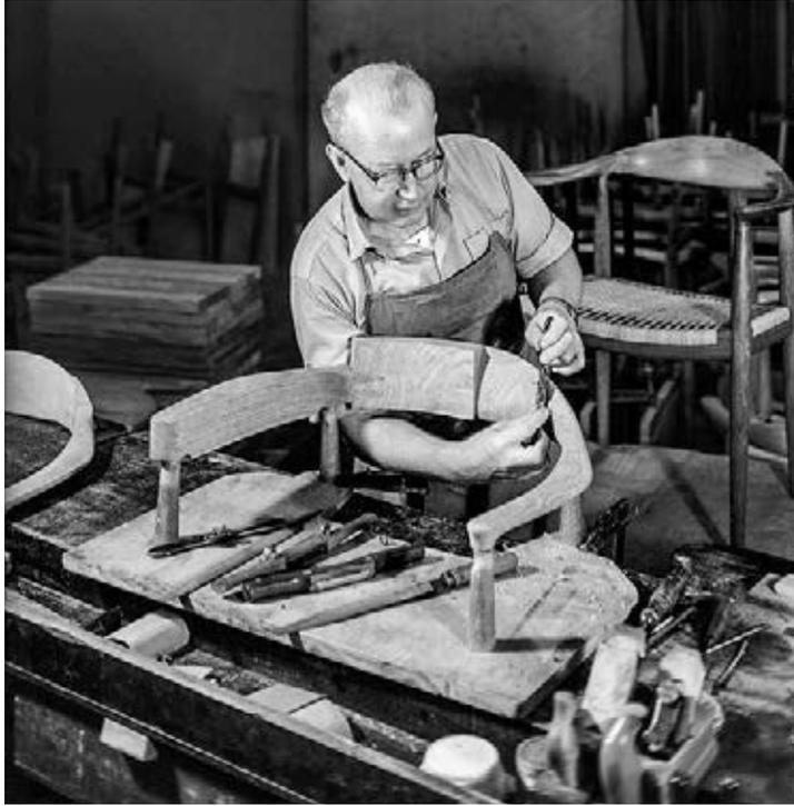
In the 1950's and 60's when the **Round Chair** were made at Johannes Hansen's workshop the shaping had to be done by hand starting with just a raw cut piece of wood. This resulted in many different 'versions', some of which varied significantly from the original design both in terms of shape, strength and comfort.
